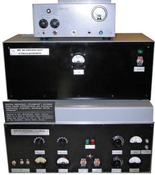
Front panel view of the three units of the replica Blyskawica transmitter: Modulator unit (top), AC mains 1500V HT power unit (centre) and actual transmitter (bottom).
